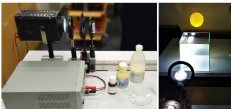
Fig. 2: The set-up of the experiment with a xenon lamp, a diaphragm and an achromatic lens. In between a filter holder is placed. The aquarium is illuminated and the transmitted light is shown on a wall.
