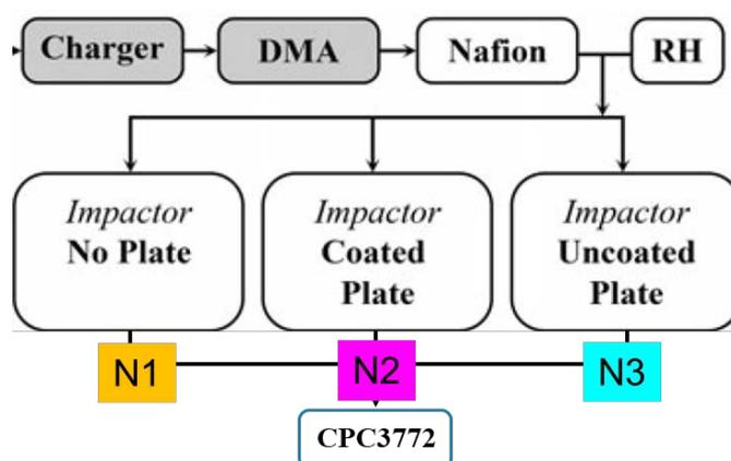
Fig 1. Schematic of the three-arm impactor
