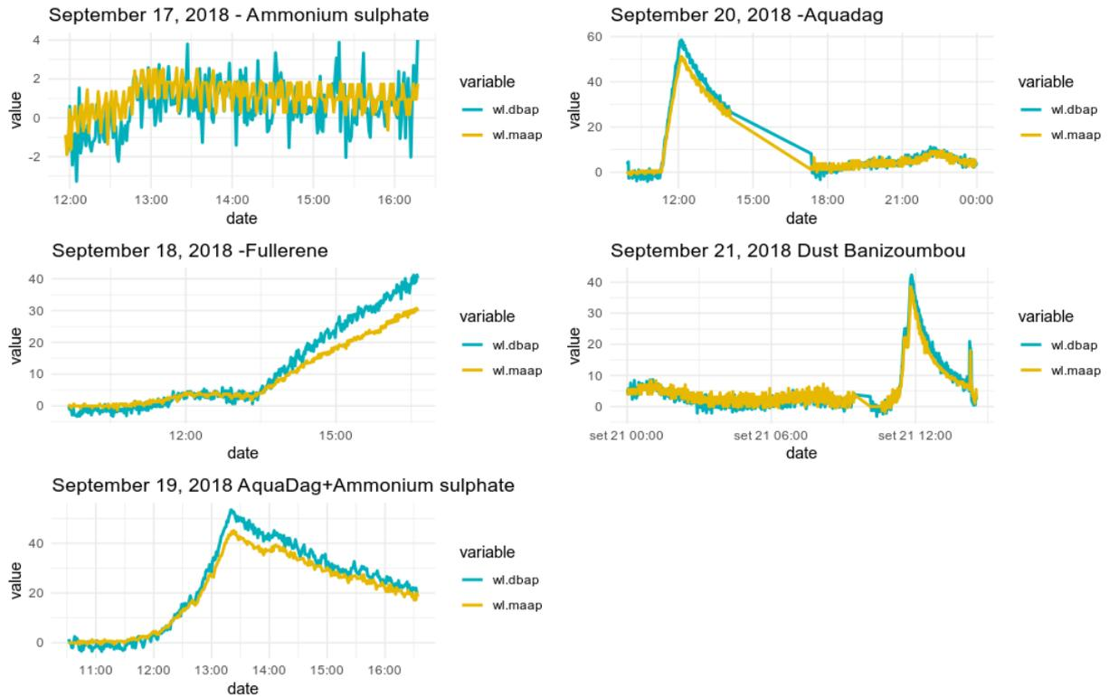
The comparison shows that there is a general good agreement in the observations by the two instruments. The DBAP and the MAAP agree in representing the temporal changes of absorption among experiments. However, the noise on the DBAP measurements for zero-absorption aerosols (ammonium sulfate, left top panel) is higher than in the MAAP measurements, affecting the limit of detection of the measurements.
