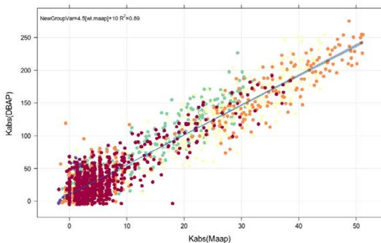
The different days are represented by varying colors. A linear fit between the two dataset can be done. Despite an evident dispersion, especially in data close to zero, the correlation is very good ( $R^2=0.88$ ). However, the DPAB data overestimate by about a factor 5 the absorption measured by the MAAP. The best fit line is represented by a slope of 5.1 and an intercept of 4.4
