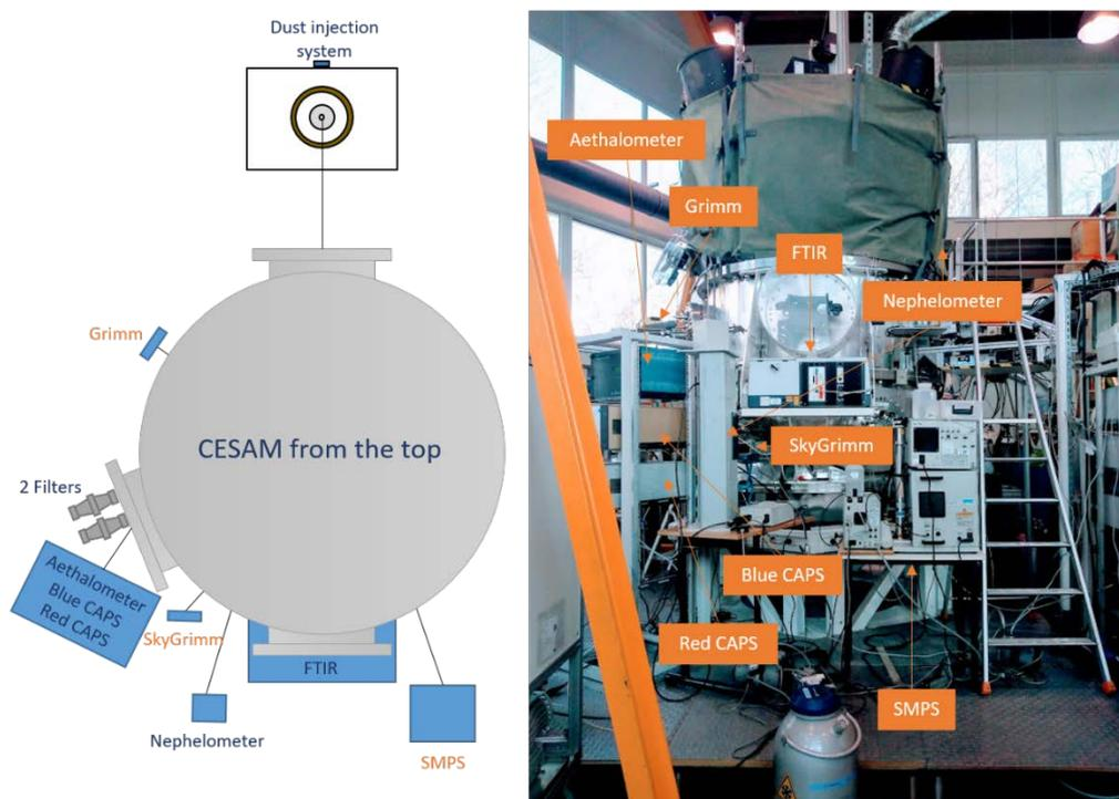
Figure 2. Schematic diagram of the chamber and the instrument setting
