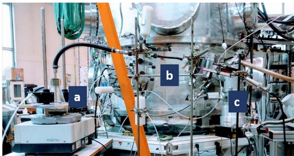
Figure 3. PM<sub>10</sub> collection system. a) Injection area, b) Resuspension chamber, c) Sampling apparatus
