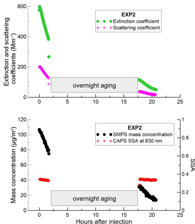
**Figure 3.** (Top) Aerosol extinction and scattering coefficients and (bottom) aerosol mass concentration and single scattering albedo (SSA) versus time for EXP2. Optical data are at 630 nm. Data are not corrected for dilution
