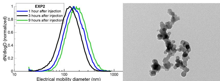
**Figure 1.** (Left) Size distribution measured during EXP2 after 1 hour from injection in CESAM and 3 and 9 hours later. (Right) MET image of the fresh soot aerosols (within one hour from injection) in CESAM for EXP2.
