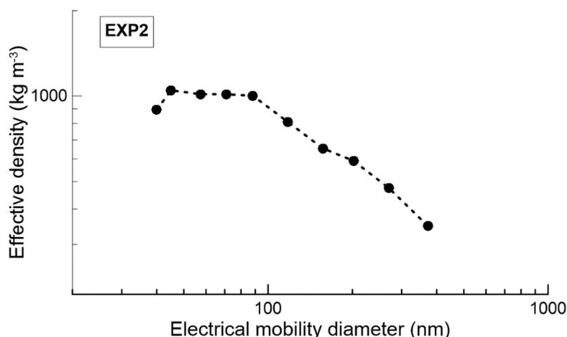
**Figure 2.** Effective density versus electrical mobility diameter for generated BC aerosols during EXP2.
