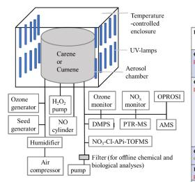
Figure 1 Experimental setup
