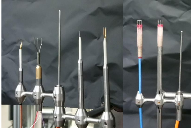
Fig.1. Thermometers participating in the experiments within the project (from left to right): UFT-2-B, UFT-M, PT100, ColdWire (Dantec Dynamics 55P71), UFT-2-A, UFT-2-0, UFT-2-0, PT100.
