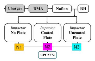
Fig 1. Schematic of the three-arm impactor
