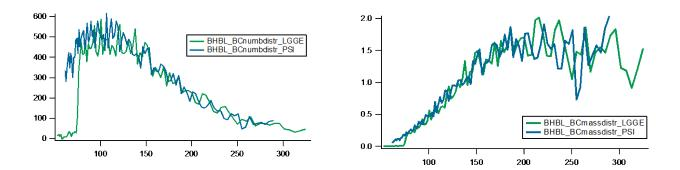
The scattering size distribution is consistent only in diameter range from 250 to 400 nm, that could be due because of the different detector used (HG in LGGE vs Split in PSI).
