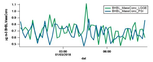
Both Number and Mass BC size distributions fitted very well between two instruments, as shown in the following graphs.
