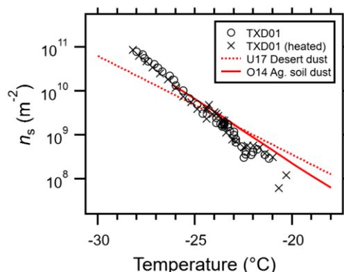
**Figure 1.** Ice nucleation active surface-site density,  $n_s$ , of TXD01 as a function of  $T$ . A comparison of non-heat-treated sample (circle marks; TXDUST01\_07-08) to heated-sample (cross marks; TXDDUST01\_03-04) is shown. Two reference lines are adapted from *Ullrich et al.* (2017; U17) and *O'Sullivan et al.* (2014; O14).
