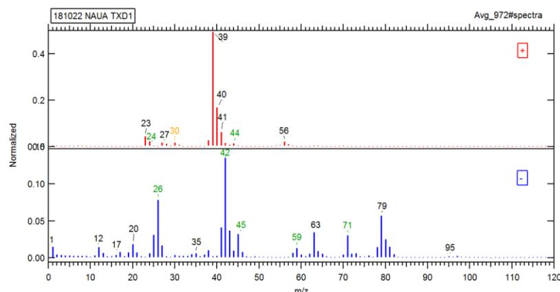
**Figure 1.** Average positive (top) and negative (bottom) ion mass spectra for 972 single TXD1 particles after laser ablation and ionization at 193 nm.
