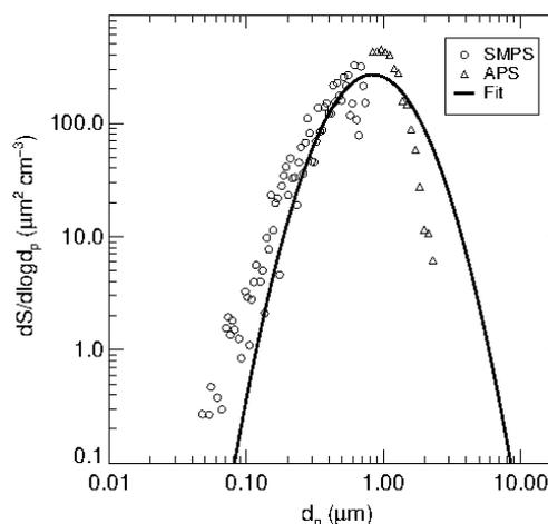
**Figure S1.** Surface area size distribution of TXD01 (from the experiment TXDUST01\_07) measured by a combination of SMPS and APS. We assume a particle density of 1.0 g cm<sup>-3</sup> and a unit dynamic shape factor.
