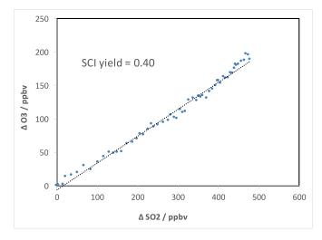
Figure 2: Loss of  $SO_2$  against loss of  $O_3$  from the same experiment as shown in Figure 1. The gradient of the plot gives the total SCI yield (Equation E1).
