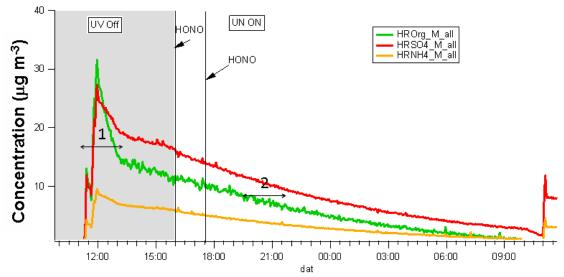
**Figure 1.** AMS results of a typical experiment with Norpinic acid and ammonium sulfate particles. The first phase is the characterization of the particles in the dark. HONO was injected and the lights were turned on at 16:00 for the chemical aging phase.
